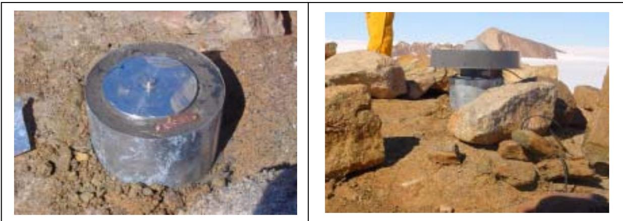
**Figure 3. Photo of AUS351 Station Mark and GPS Choke Ring Antenna**
