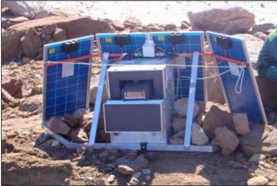
**Figure 4. Solar Panel and GPS warm box set up at AUS 351**
