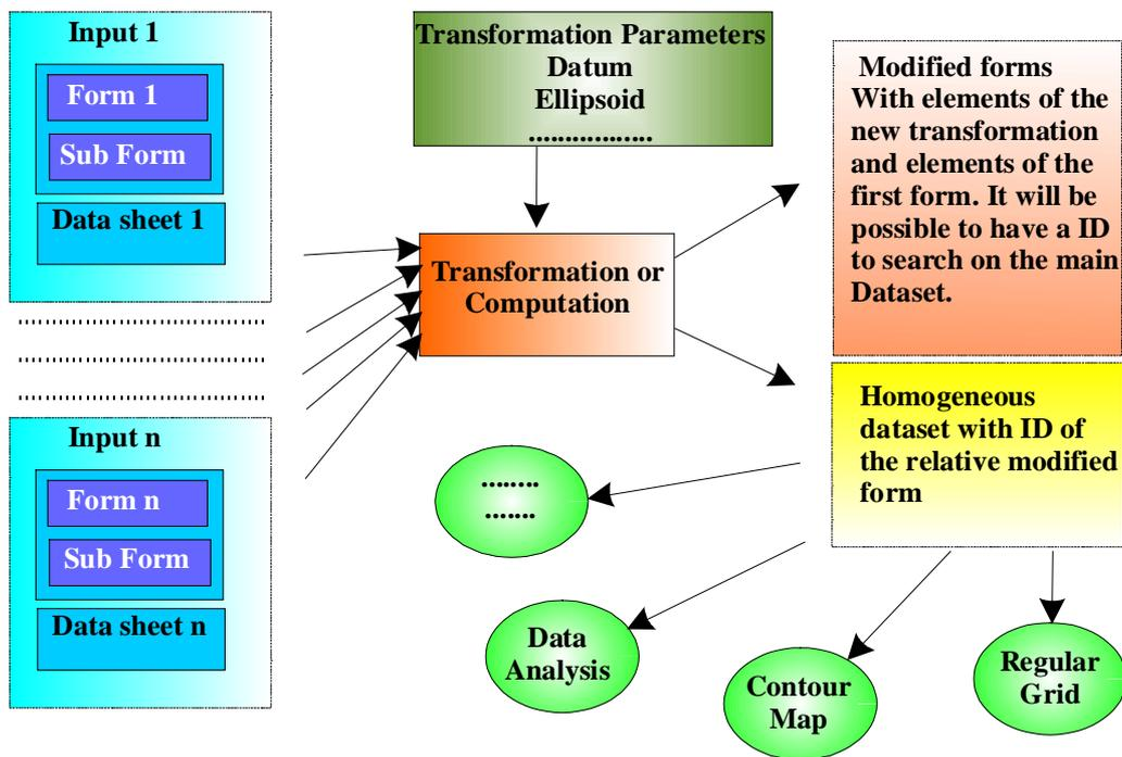
Fig. 2. - Main Scheme of the DBMS for Geodesy
