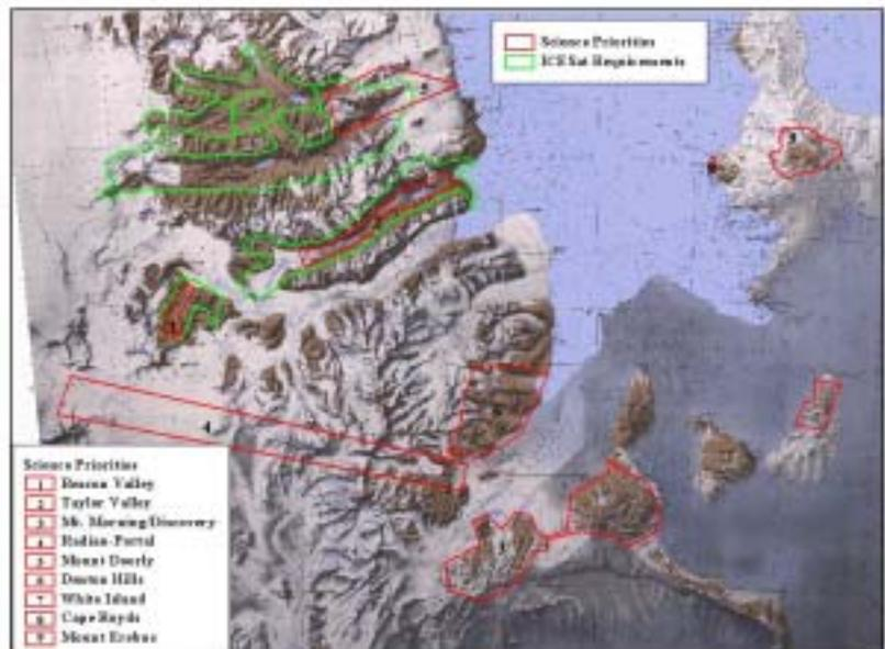
Twin Otter aircraft and nearly a week of waiting for the weather to clear, data collection began December 18 and continued through Dec 31, 2001. They collected elevation data with 1-5 meter horizontal sampling and 10-50 cm vertical resolution for the selected areas from priority 1 through 9 as shown below. Vertical resolution varied based on area requirements.
