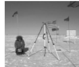
Coordinated with the Raytheon surveying engineers for the 2001-2002 construction season at South Pole, a high accuracy geodetic survey was performed. Two existing and two new stations of the SP-GEONET were occupied. Station AMUN was the reference station for the resultant coordinates. One of the two new stations was located on the roof of the new elevated structure (ELST) and the second station was located on the roof of building for the MARISAT RF equipment (RFBD).
