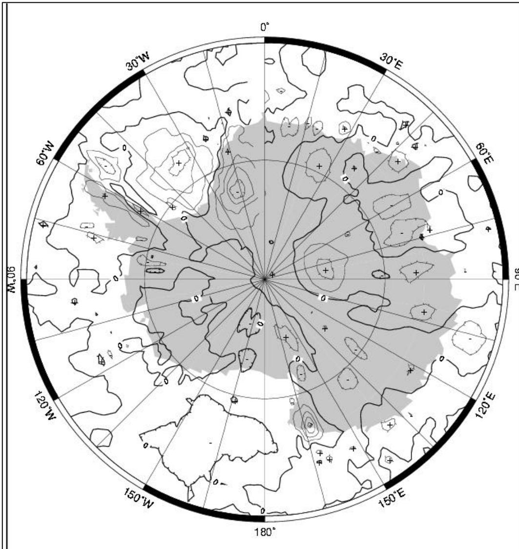
Figure 2: EGM96 minus OSU91 geoid ellipsoid separations (1 metre contour interval)
