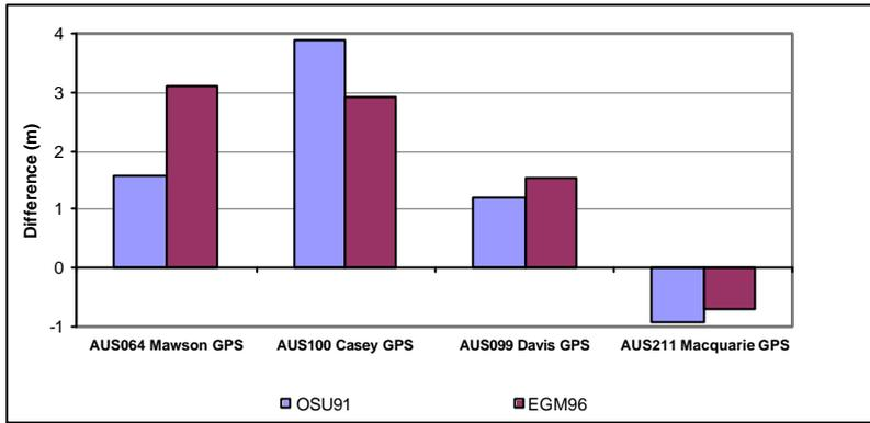
Figure 1: Comparison of Geometric and gravimetric geoid-ellipsoid separations at AUSLIG GPS stations, using OSU91 and EGM96
